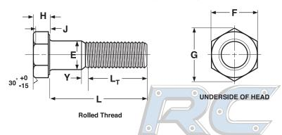
±Length of a cap screw is measured from the underhead bearing surface to the extreme end of the screw.
