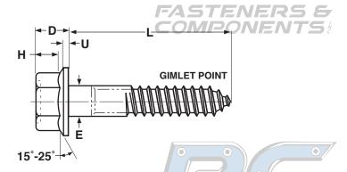
Length of a hex flange lag screw (L) is measured from the underhead bearing surface to the extreme end of the screw.
