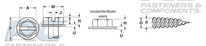
Head dimensions of self-piercing screws differ from those of standard tapping screws.
